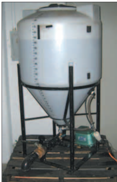
This compost tea brewer will make 110 gallons. The brewer has an air pump, an air diffuser inside the tank, and a heater.
